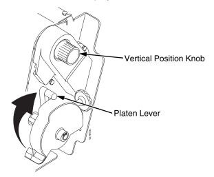
Figure 10. Raising the Platen Lever
